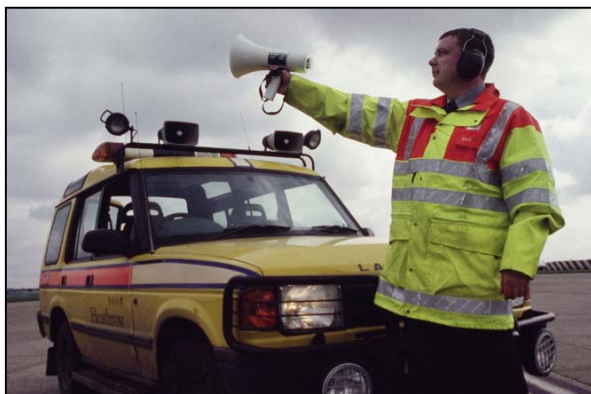
A mobile patrol equipped with scaring devices such as pyrotechnics and distress calls is the most efficient way to detect and disperse birds.
