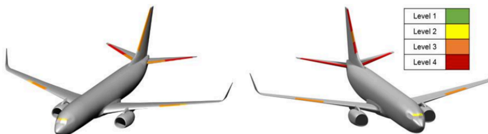
Figure 27 Damage severity levels to commercial transport jet airframe
