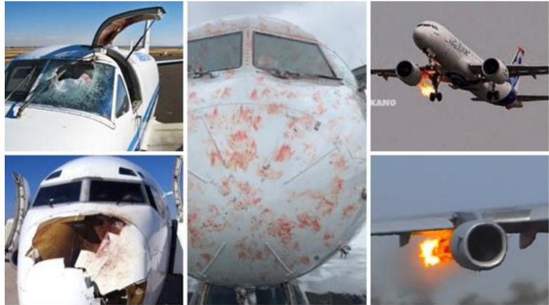
Figure 1 Bird strike damage to the aircraft
