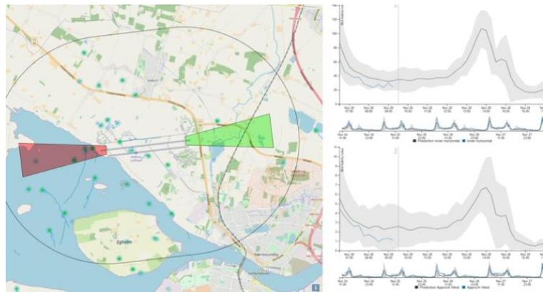
Figure 3 Take-off or approach in opposite direction if risk is lower at one runway end and weather and traffic permits. Source: Ascend
